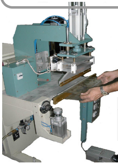
Sheet Welding with Sleeveboard under-electrode and Cylinder as mechanical Support
